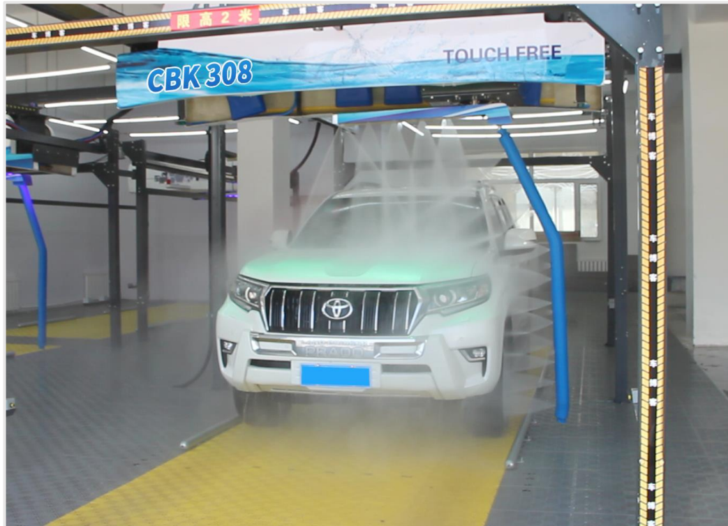
308 Touchless car wash equipment
