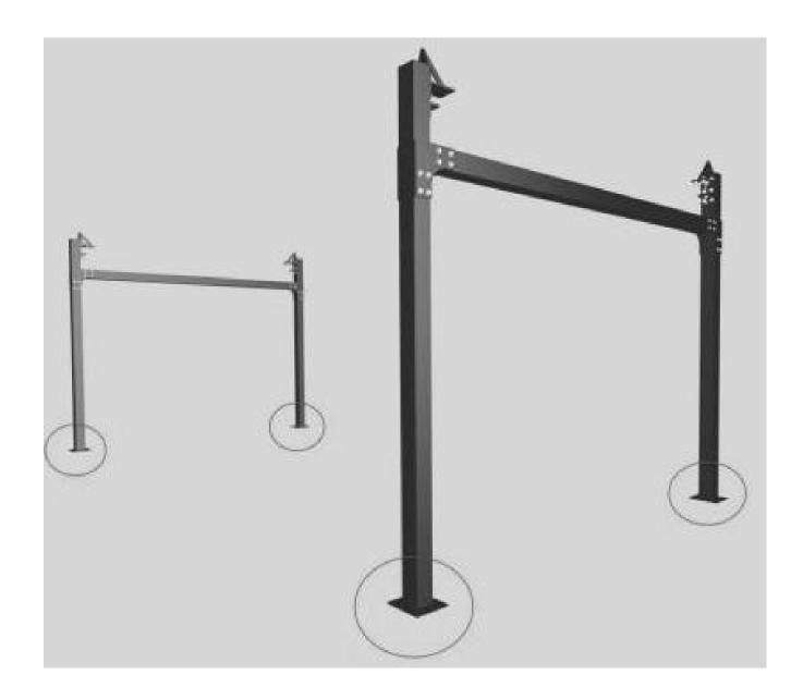
3. When measuring the position of frame, please take the inner boundary of the column as the benchmark.
